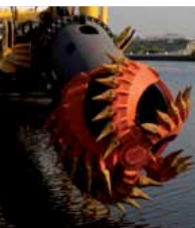
HEAVY DUTY CUTTER A heavy duty cutter can be mounted for consolidated soils.
