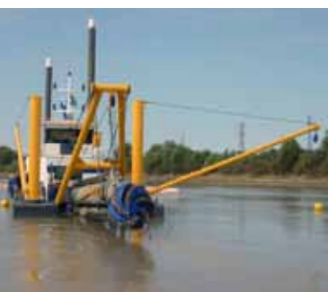
ANCHOR BOOMS Anchor booms, made of heavy gauge pipe, are used to swiftly reposition the anchors.
