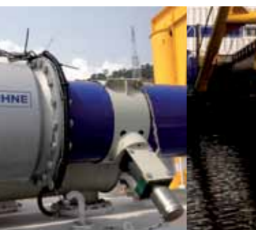
DREDGING INSTRUMENTATION Production measurement system visualizes the real time production on a cross needle screen and logs this production using counters.
