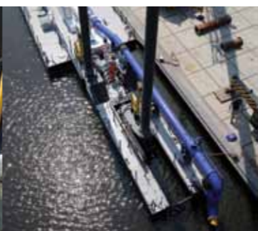
SPUD CARRIAGE PONTOON A spud carriage pontoon can be added to the main pontoon to increase efficiency
