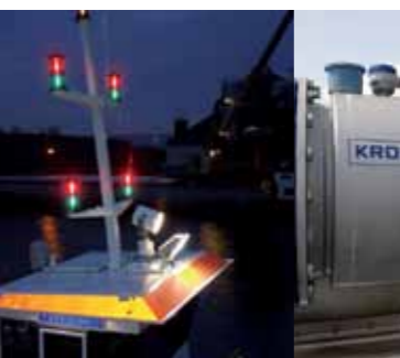
NAVIGATION LIGHTS A foldable mast with navigations lights can be added to the operating cabin.
