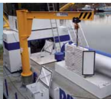
JIB CRANE A jib crane can be mounted on the portside aft pontoon to handle pump parts and spares.
